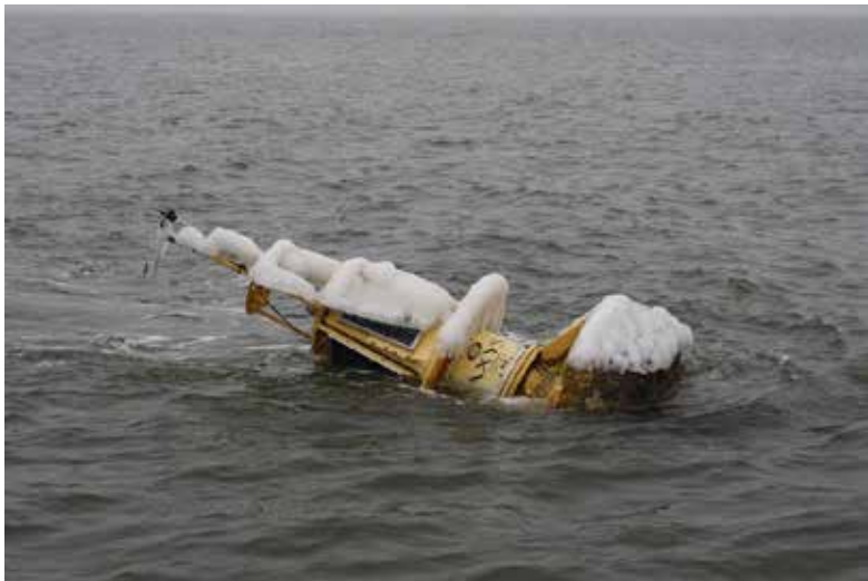
Figure 3: The impact of ice loading on a CBIBS buoy like this one in the Potomac River can confound measurements and destroy sensors. Ice floes can also drag the buoys out of position. (Photo courtesy of NOAA)
